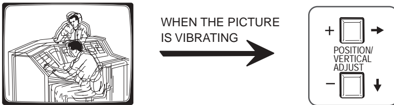
Figure 30. Vertical Picture (Vibration) Adjustment
